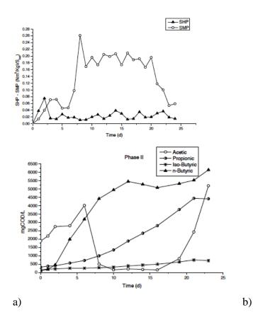
**Figure 17.** a) SHP and SMP trends with digestate recirculation, at OLR 30 kg VS m<sup>-3</sup> day<sup>-1</sup>; b) acetic, propionic and butyric acid profile, second phase with digestate recirculation, at OLR 30 kg VS m<sup>-3</sup> day<sup>-1</sup>
