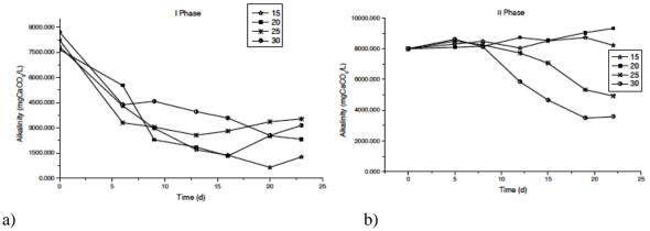
**Figure 12.** a) First phase alkalinity comparison, supernatant recirculation; b) second phase alkalinity comparison, supernatant recirculation.
