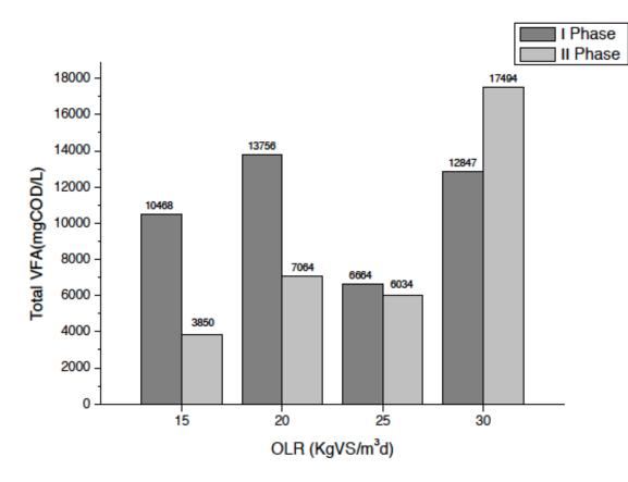
Figure 19. Total VFA for all the OLR tested with digestate recirculation
