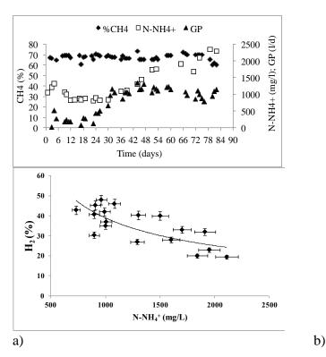
**Figure 28.** a) Effect of ammonia concentration in the anaerobic digestion reactor; b) Effect of ammonia on biohydrogen production in dark fermentation reactor.
