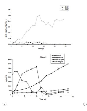
**Figure 16.** a) SHP and SMP trends with digestate recirculation, at OLR 25 kg VS m<sup>-3</sup> day<sup>-1</sup>; b) acetic, propionic and butyric acid profile, second phase with digestate recirculation, at OLR 25 kg VS m<sup>-3</sup> day<sup>-1</sup>
