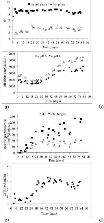
**Figure 26.** a) pH profile of both reactors; b) alkalinity concentration in anaerobic digestion reactor; c) total gas and hydrogen specific gas production in the first phase; d) gas production rate in second phase reactor.
