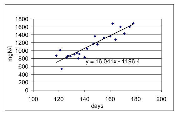
Figure 25. Rate of ammonia accumulation in second phase reactor Run III
