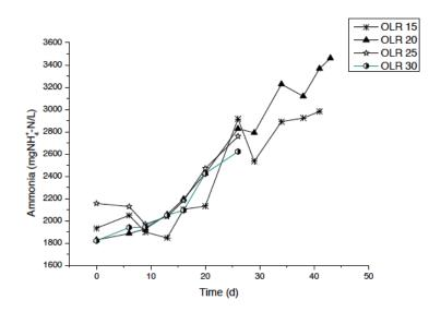
Figure 20. Ammonia accumulation during the second phase with digestate recirculation
