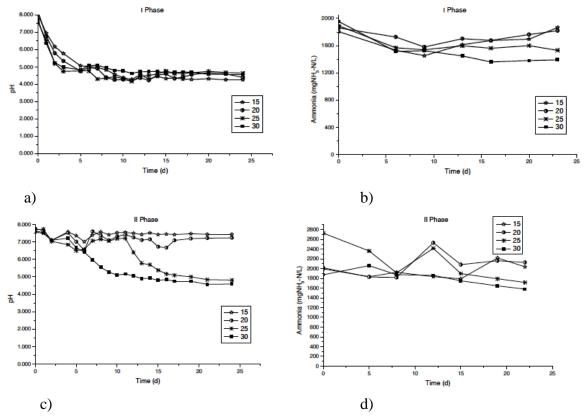
**Figure 13.** Supernatant recirculation trial, a) first phase pH; b) first phase ammonia, c) second phase pH; d) second phase ammonia
