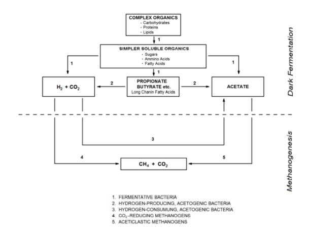
Figure 1. Separation of the AD stages in a two-phase system
