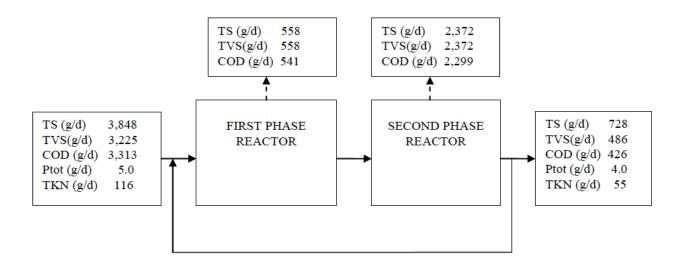
Figure 24. Mass balance of Run IIIa
