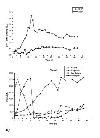
**Figure 15.** a) SHP and SMP trends with digestate recirculation, at OLR 20 kg VS m<sup>-3</sup> day<sup>-1</sup>; b) acetic, propionic and butyric acid profile, second phase with digestate recirculation, at OLR 20 kg VS m<sup>-3</sup> day<sup>-1</sup>.
