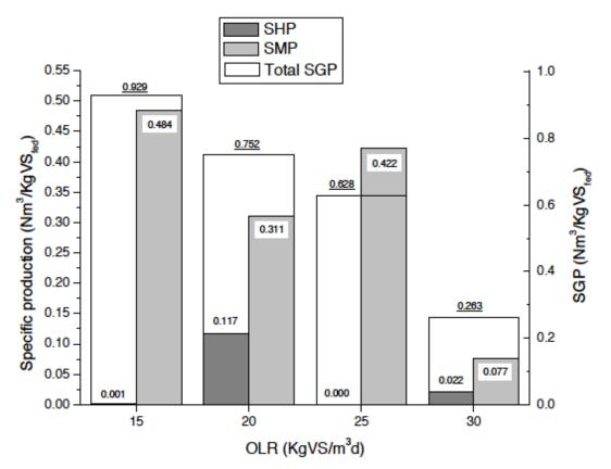
Figure 18. Specific Gas Productions for all the OLR tested with digestate recirculation
