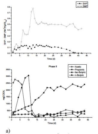
**Figure 14.** OLR 15 kg VS m<sup>-3</sup> day<sup>-1</sup>. a) SHP and SMP trends with digestate recirculation; b) acetic, propionic and butyric acid profile, second phase with digestate recirculation
