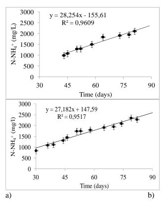
**Figure 27.** Ammonia accumulation rate a) in dark fermentation reactor; b) in anaerobic reactor.
